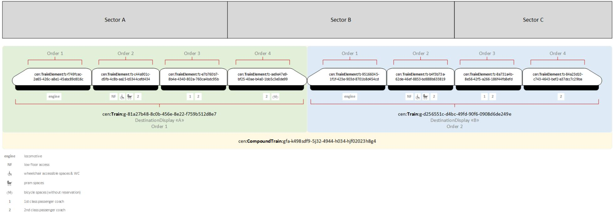
**Figure 14 - Illustration of the train formation at the first call («..StopPoint:998375543» / Order «10») with the vehicle features and the coaches mapped to sections on platform 2 («...Quay:76007252:11»)**
